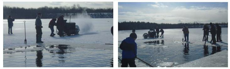
For 26 years, ice has been harvested on Tobyhanna Mill Pond No. 1. This year it was harvested on a beautiful 20° Saturday in January. In years past, a Ford Model A or T engine powered ice cutting machines with a large 36″ circular saw blade. In these photos, you see the machine cutting the ice after it has been scored in a grid pattern. If ice is deeper than the saw blade, cakes are separated with a spud bar or manually with an ice saw.
